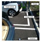
Figure 7: Eavesdropping from the next parking bay (site G), more than 4 metres away on the other side to the charging cable. In this arrangement 91.8% of messages were received successfully.
