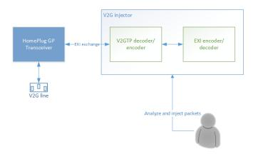
We can intrude a HPGP network, and analyse/decode/encode/inject V2G data
