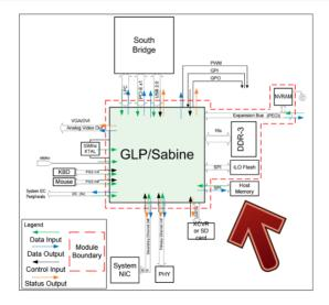
iLO is directly connected to the PCI-Express bus.
