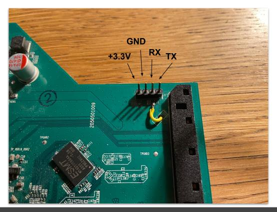
A good logic analyzer will help finding the right parameters to decode the serial communication
