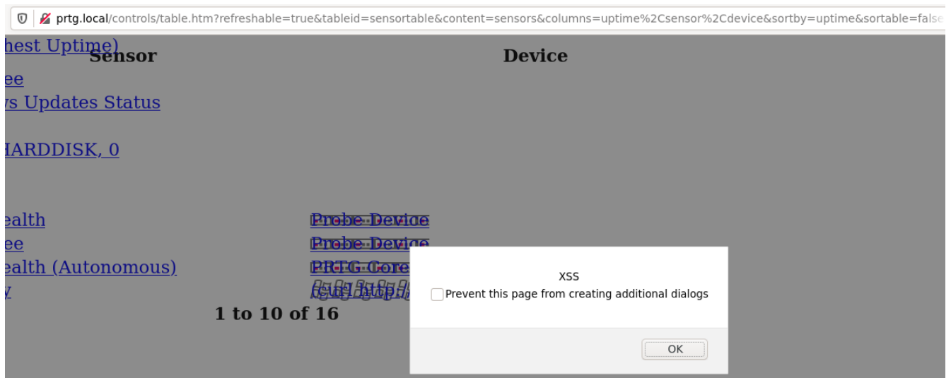
Figure 2: Reflected XSS vulnerability in /controls/table.htm .
