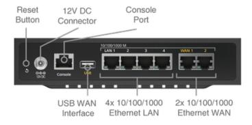
This port, ttyso, is also configured to output kernel logs.
